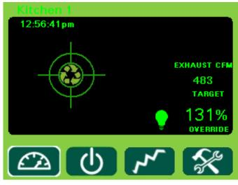
This is the Dashboard Window for Kitchen1. The Dashboard displays the Kitchen1 operational parameters. The Kitchen1 name can be changed through the setup screen with a password.
