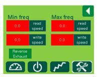
Touch read speed for Min freq. The field will turn pink for several seconds and then display the current minimum operating frequency on the drive.
