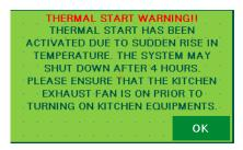
The TruFlow Lite will automatically turn on the exhaust and supply fans when a threshold temperature under the hood is reached.
