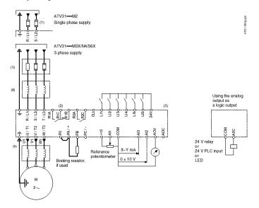
NOTE: The line supply terminals are shown at the top and the motor terminals are shown at the bottom. Connect the power terminals before connecting the control terminals. Install surge suppressors on all inductive circuits located near the drive controller or coupled to the same circuit.
