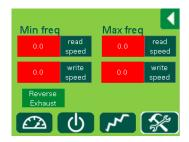
Touch read speed for Min freq. The icon will turn pink for several seconds, then change to the minimum frequency on the drive.
