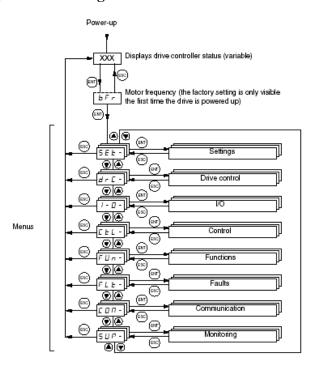
The following figure illustrates how to access parameters and assign their values. To store the parameter value, press the key. The display flashes when a value is stored.
