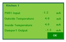
PXR1 Input is the value being received from the variable speed drives – it represents the current operating speed of the fans.
