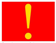
When a message that requires immediate attention or action occurs, the screen will change to red with a yellow exclamation mark. These types of alarm include certain drive errors where the VFD cannot reset automatically, and catastrophic equipment failures (exhaust fan or makeup air unit not running).
